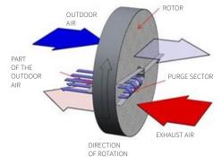
The main influence on the correct function of the purge sector is the location and pressure ratio of the fans in the HVAC unit. The most suitable position of the rotary heat exchanger in the HVAC unit is the suction side of both the supply and exhaust fans and the countercurrent flow.
